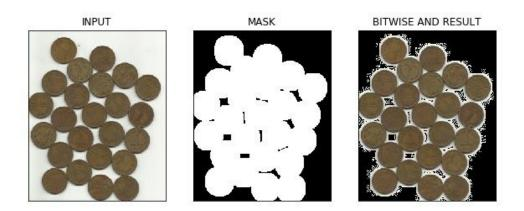
In the above figure, we can see an input image and its segmentation mask calculated using the Watershed algorithm. Further, we have applied the bitwise 'AND' operation to remove the background from the image and extract relevant portions from the image. Pretty awesome stuff!
