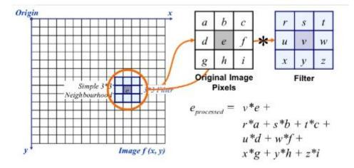
Gaussian filtering is also used for image blurring that gives different weights to the neighbouring pixels based on their distance from the pixel under consideration.
