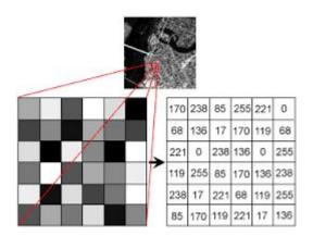
Every number represents the pixel intensity at that particular location. In the above image, I have shown the pixel values for a grayscale image where every pixel contains only one value i.e. the intensity of the black color at that location.
