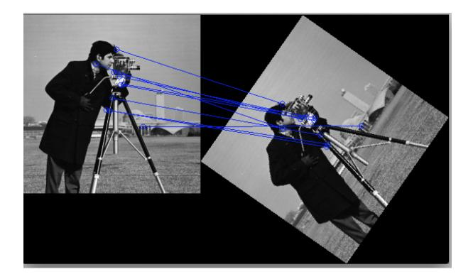
In the above image, we can see that the keypoints extracted from the original image (on the left) are matched to keypoints of its rotated version. This is because the features were extracted using SIFT, which is invariant to such transformations.
